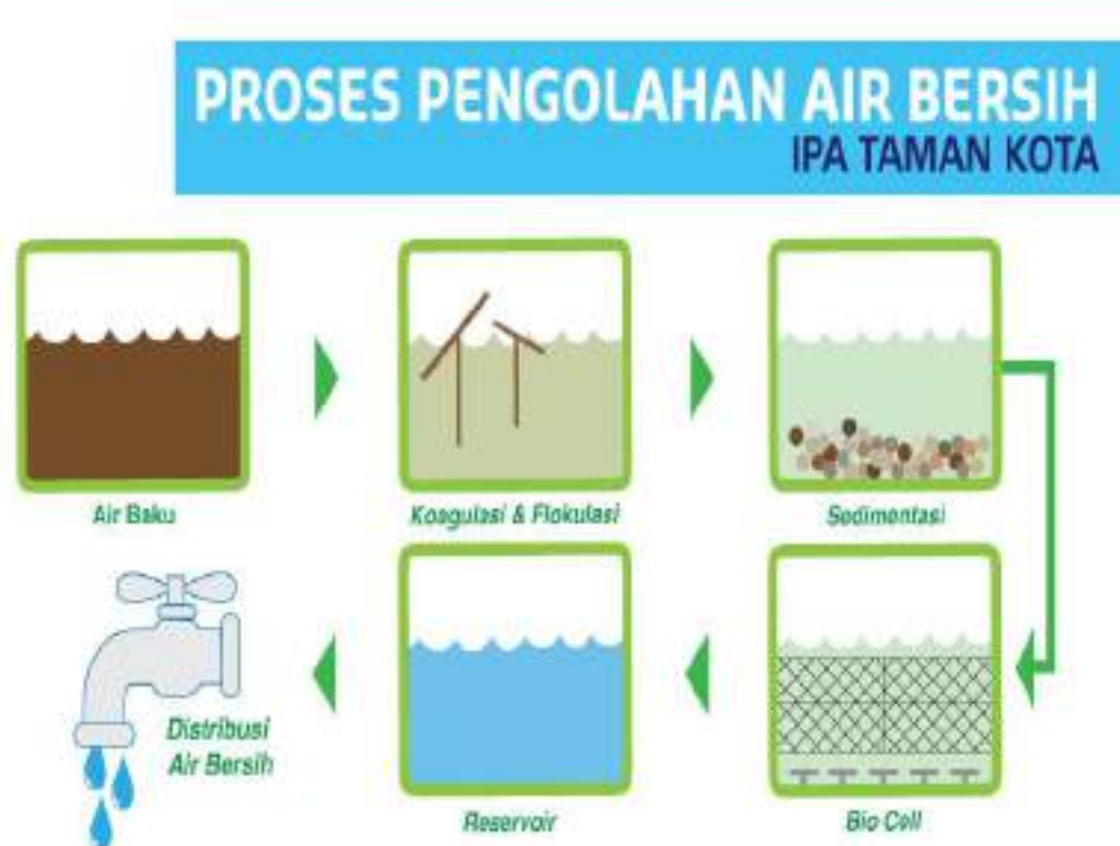
Gambar 1.37: Proses Pengolahan Air Bersih https://www.google.com/search?q=Gambar+pengolahan+air
